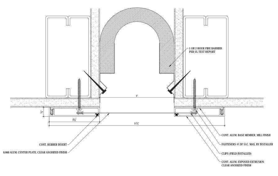
NOTE: 1 HOUR CONSTRUCTION INDICATED 2 LAYERS OF GYPSUM BOARD FOR 2 HOUR CONSTRUCTION
